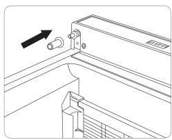
4. Reverse the door and hang it onto the left upper hinge.
